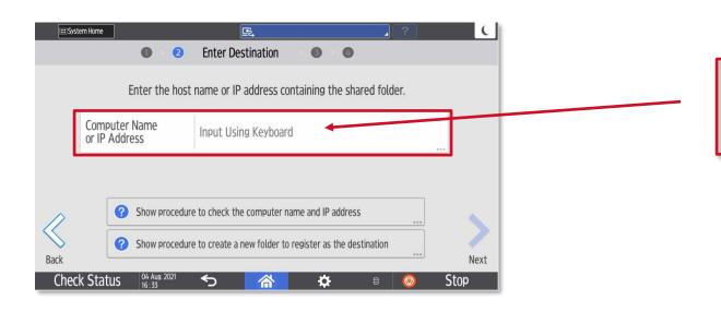
Add the IP address or the hostname for the destination computer here, using the pop-up keyboard.
