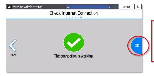
If all is well, touch **OK**. If the connection fails, please check IP address, Gateway and Subnet Mask are correct and test again.
